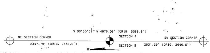
(c)(d)(e) Plan view of corner with ties to at least 4 witness monuments. If in disagreement with previously established corner, show the distances between the two corners and also indicate the ties to the
