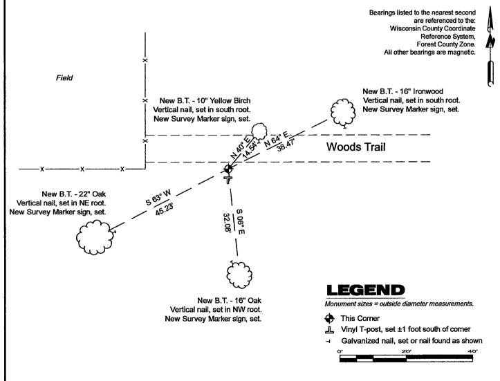
A-E 7.08(3)(e) 1858 Surveyor set a post, 1965 Surveyor found an iron pipe and replaced it with a 1" diameter galvanized iron pipe with an aluminum cap, 2004 Surveyor found a 4" dia. alum. mon. I found a 1.3" diameter galvanized iron pipe monument, with a 4" diameter Jeffrey De S 2658
