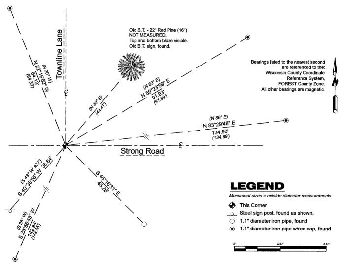
A-E 7.08(3)(e) 2008 Surveyor set a "Survey Spike", 2012 Surveyor found a "nail". I found the shaft of a survey spike (or nail) and witnesses.
