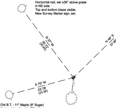
Horizontal nail, set in SE side. Top and bottom blaze visible. Old B.T. sign, found.
