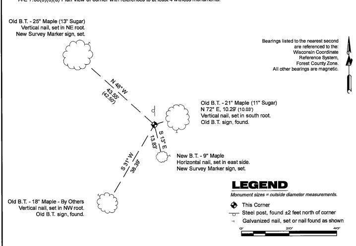
A-E 7.08(3)(e) 1857 Surveyor set a post, 1975 Surveyor found a cedar post and set a 2 1/2" aluminum monument, 1995 and 2024 Surveyors found the same. I found 2.4" diameter aluminum pipe monument with a 3.25" diameter aluminum cap stamped to identify the corner location in 2025.
