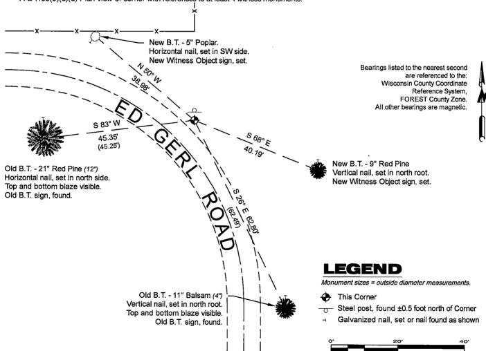
A-E 7.08(3)(e) 1857 Surveyor set a post, 1985 Surveyor set a 2 1/2" diameter aluminum pipe monument, with aluminum cap stamped to identify corner, 2019 Surveyor found a monument. I found a 2.25" diameter aluminum pipe monument with a 3.25" diameter aluminum cap stamped to identify the corner in 2024.
