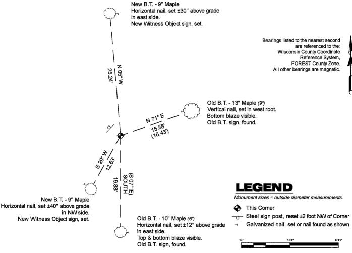
A-E 7.08(3)(e) 1857 Surveyor set a post, 1985 Surveyor found a 2 1/2" diameter aluminum pipe monument, with a aluminum cap stamped to identify corner, 2016 Surveyor found similar monument. In 2024, I found a 2.25" diameter aluminum pipe with a 3.25" diameter stamped aluminum cap stamped to identify corner location.
