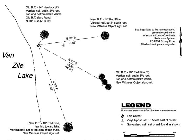
A-E 7.08(3)(e) 1857 Surveyor used a Yellow Pine as corner, 1970 Surveyor set a 2" inside diameter galvanized wrought iron pipe with brass cap stamped to identify corner. I found a 2.25" diameter galvanized iron pipe with a 3" diameter stamped brass cap in 2024.
