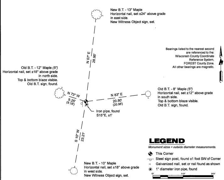
A-E 7.08(3)(e) 1857 Surveyor set a post, 1985 Surveyor found a 2" inside diameter galvanized wrought iron pipe, with a brass cap stamped to identify corner. I found a 2.25" diameter galvanized iron pipe with a 2.9" diameter stamped brass cap in 2024.
