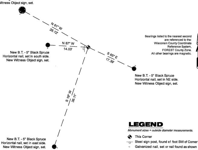
A-E 7.08(3)(e) 1857 Surveyor set a post, 1985 Surveyor set a 2 1/2" diameter aluminum pipe monument, with an aluminum cap stamped to identify corner. I found a 2.25" diameter aluminum pipe with a 3.25" diameter stamped aluminum cap in 2024.
