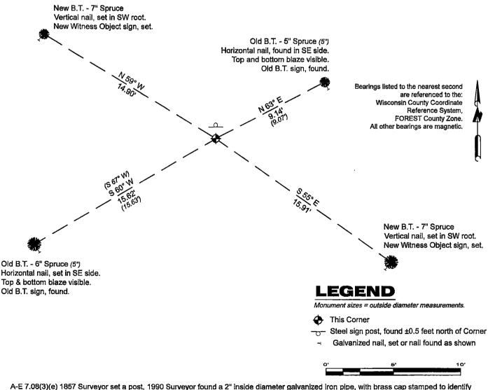
A-E 7.08(3)(e) 1857 Surveyor set a post, 1990 Surveyor found a 2" inside diameter galvanized iron pipe, with brass cap stamped to identify corner. In 2024, I found a 2.5" diameter iron pipe monument with a 3" diameter brass cap stamped to identify the corner. Jeffrey
