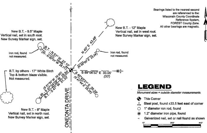
A-E 7.08(3)(e) 1857 Surveyor set a post, 2005 Surveyor found a 5/8" diameter iron rod, 2007 & 2011 Surveyor found a iron pipe. In 2024, I Settrey L S 28 Arbor V. WI SURVE found a nail with a 0.4" diameter head.
