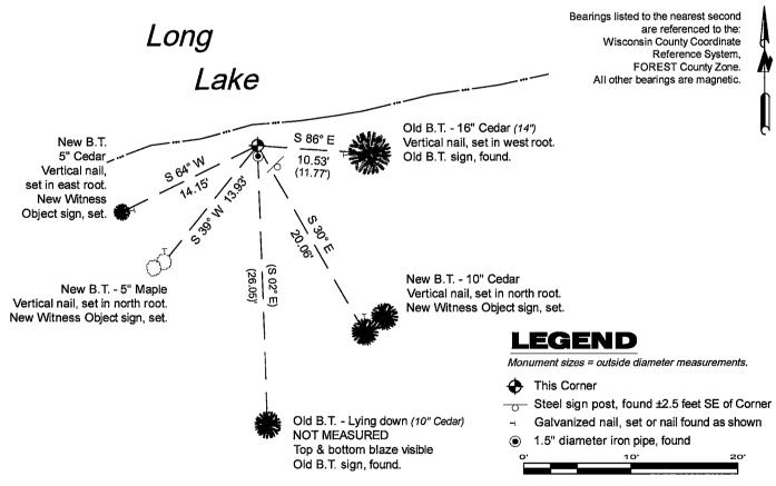
A-E 7.08(3)(e) 1858 Surveyor set a post, 1988 Surveyor found a 2 1/2" diameter galvanized iron pipe monument 36 inches long with a brass cap, 2008 Surveyor found the same. I found a 2.25" diameter galvanized iron pipe monument with a 3" diameter brass cap stamped to identify the corner in 2024.
