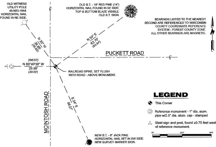
A-E 7.08(3)(e) 1865 Surveyor set a post, 1998 Surveyor found a 6" diameter concrete monument. I found a concrete monument with a 6" diameter brass cap ±1.4 feet below the road grade, and set a railroad spike at the road surface.
