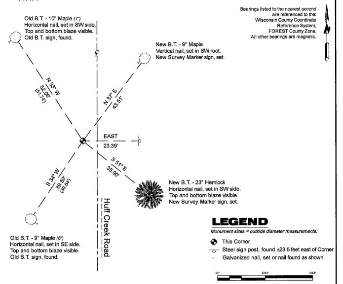
A-E 7.08(3)(e) 1865 Surveyor set a post, 1992 Surveyor set a 2 1/2" diameter aluminum pipe monument, with an aluminum cap stamped to identify corner. In 2025, I found a 2.4" diameter - damaged aluminum pipe monument without a cap. A-E 7.08(3)(f) I accept this monument in good faith as a FOUND PERPETUATED LOCATION of the corner.
