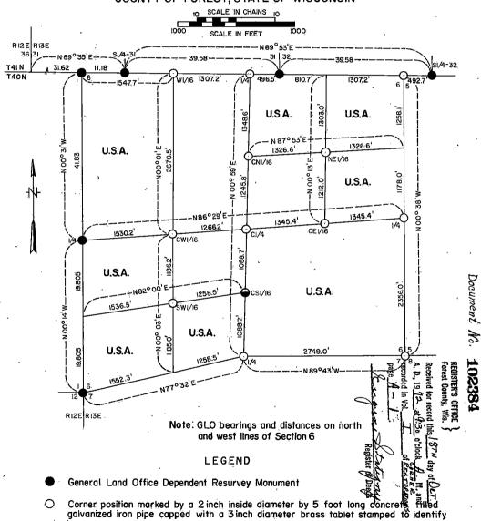
inserted 3inch diameter brass tablet stamped to identify corner.
